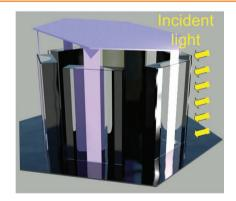
A photo-thermomechanical liquid-crystalline elastomer (LCE) nanocomposite is developed and utilized to realize artificial heliotropism. The LCE nanocomposite actuators respond to light and, in turn, drive solar cells to track the light source. Full-range heliotropism is shown in both laboratory and in-field tests under natural sunlight. A significant increase in the photocurrent output from the solar cells in the artificial heliotropic devices is observed.
