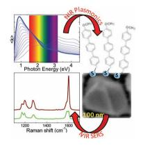
Faceted gold nanoparticles for near infrared surface enhanced Raman scattering (NIR SERS) are fabricated directly on technologically important substrates using a novel dry plasma methodology.
