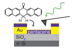
Thin pentacene films are layered with putative pentacene trap-precursors and the resulting spatial distribution of charge traps and spectroscopic trap-clearing rates under illumination are measured with time- and wavelength-resolved electric force microscopy. Pentacen-6(13H)-one efficiently generates charged traps with trap-clearing spectra resembling those of aged pentacene, while 6,13-dihydropentacene does not. It is concluded that PHO+ is the charged trap species.
