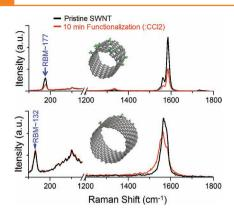
The influence of dichlorocarbene functionalization on the structural and electrical properties of individual single-walled carbon nanotubes (SWNTs) with diameters ranging from 1.2 to 2.2 nm are studied. SWNTs with small diameters are found to be functionalized more easily than those with large diameters. Furthermore, electrical conductance is preserved for most SWNTs, while effective bandgap variations are generally observed.
