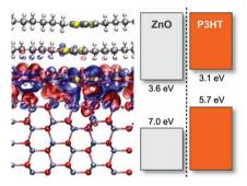
Using first-principles calculations the energy-level alignment of organic/inorganic solar cell interfaces based on ZnO and poly(3-hexylthiophene) (P3HT) is investigated. The interfacial charge transfer is shown to increase the ideal open-circuit voltage with respect to the electron-affinity rule by 0.5 V. The findings suggest that that there is room for improving the efficiency of these devices by tailoring the semiconductor/polymer interface at the nanometer-scale.
