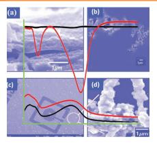
Nanocomposites of chiral poly(fluorene-alt-benzothiadiazole) (PFBT) dispersed in achiral SU-8 photopolymer show dramatic enhancement of circular dichroism (CD). Thin films with a 1/20 to 1/40 ratio of PFBT/SU-8 have maximum CD values up to 75 times that of a pure chiral PFBT film of equal optical absorbance. This is attributed to supramolecular organization of chiral polymer fibrils.
