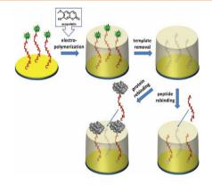
Surface imprinting of the C-terminal peptide epitope of cytochrome c can be achieved by forming an ultrathin polymer film of comparable thickness of the peptide template. The imprinted film shows selective binding to both the peptide template and target protein. The film is directly prepared on the electrode surface, making this strategy very useful for sensor applications.
